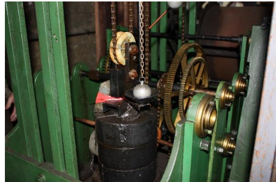
Earlier auto-winding, showing additional weight being added with sticky tape – not a proper solution.
